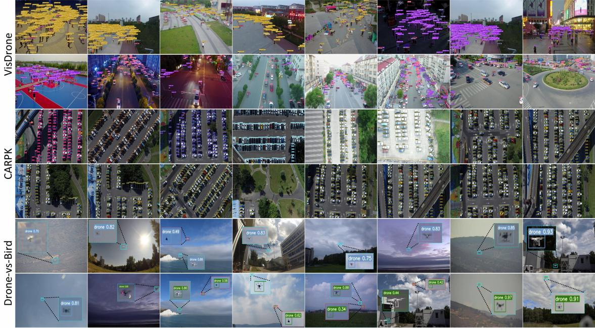
Figure 3. The visualization results of FGHDet on the VisDrone (1<sup>st</sup> and 2<sup>nd</sup> row), CARPK (3<sup>rd</sup> and 4<sup>th</sup> row), and Drone-vs-Bird (5<sup>th</sup> and 6<sup>th</sup> row) test sets, using different colors to differentiate between the different classes, are still effective in scenarios with dense distributions and small objects.
