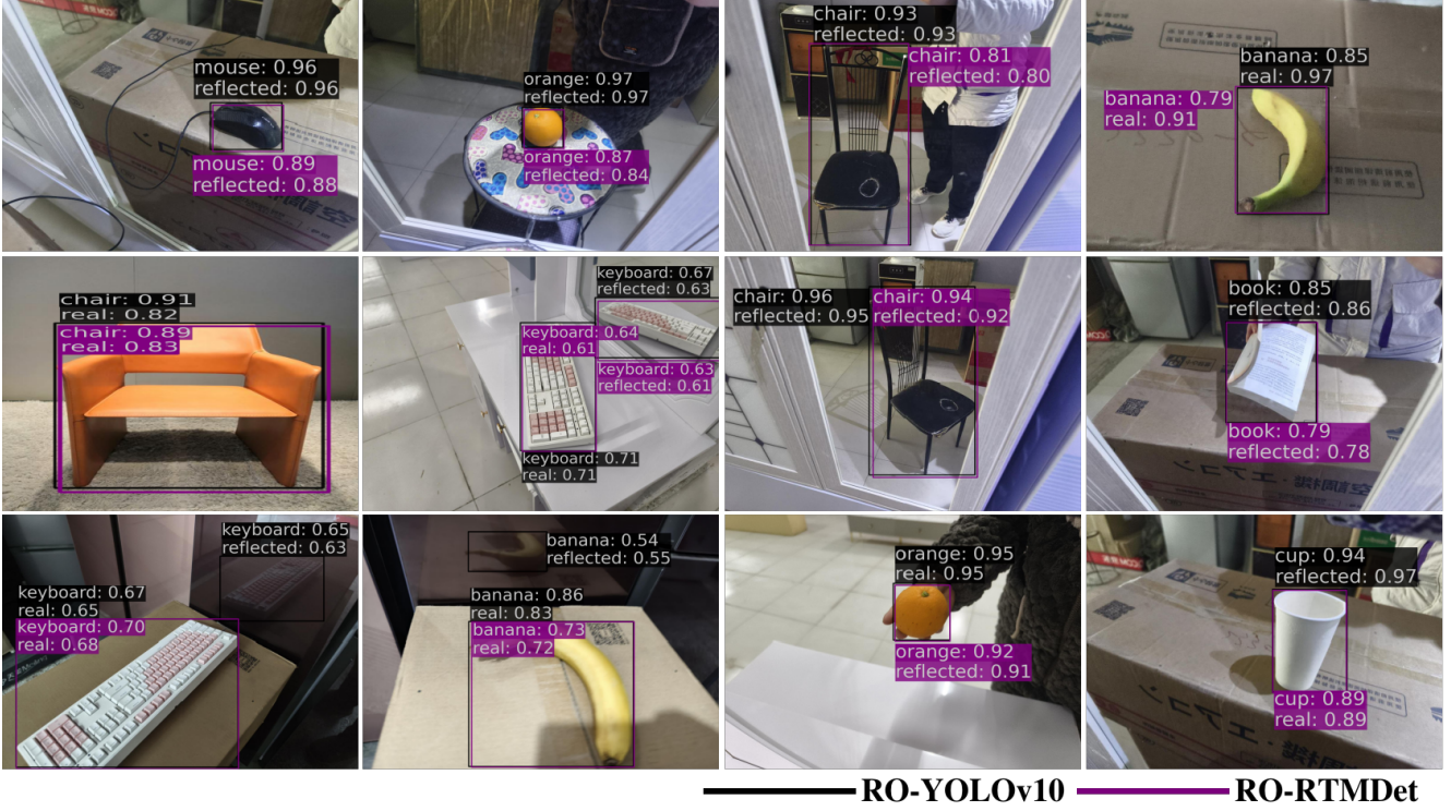
Figure 9: A qualitative evaluation was conducted on 12 samples from ROD dataset. The first two rows display examples accurately predicting the nature of objects using RO-YOLOv10 and RO-RTMDet detectors, while last row shows error detection results generated by these two detectors. Note that the predicted bounding box, object category, object nature, and the corresponding scores have been marked in the images.
