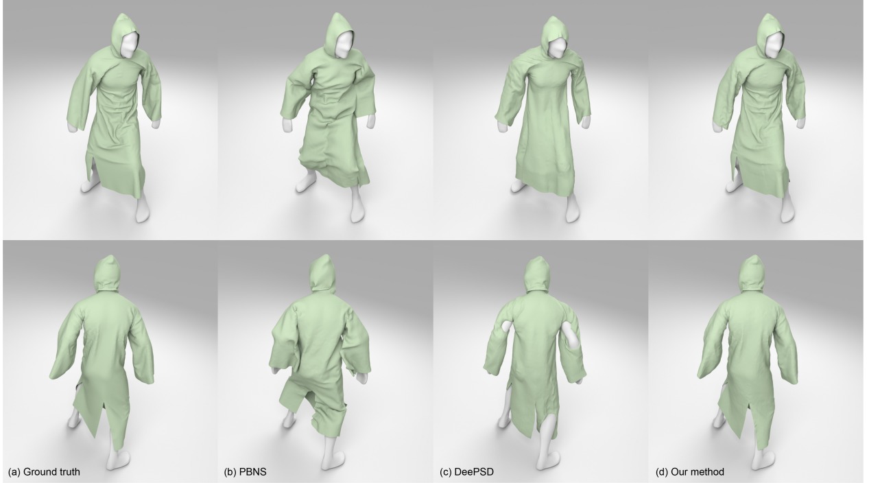
Figure 10. Comparison of results between our network and previous methods. The first column is the ground truth of the deformed cloth. The second and third columns are the results of [2] and [3]. The last column is the result of our method. The top and bottom rows are the front and back views of the deformed predictions.
