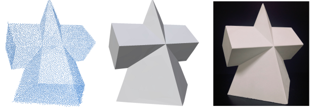
Figure 9. Reconstruction result (middle) on a real scanned point cloud (left) which is obtained by scanning the object (right) with EinScan-SP 3D scanner.
