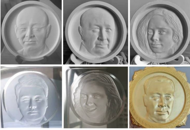
Figure 11. Reliefs fabricated by NC machining with different material. Top: plaster. Bottom-left: acrylic. Bottom-right: copper plated with gold.
