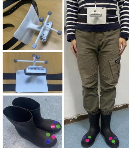
Figure 2: The prototype of our waist-mounted capturer. The extended branches fixed with reflective markers are used to collect the training data. They can be removed after the training stage.
