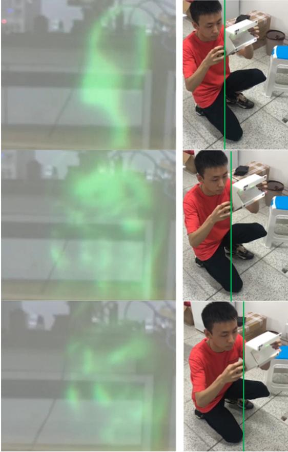
Figure 8: Experiment of visualizing CT images with an AR experience. When the user moves forward or backward (the right column), the user can see different CT images on their corresponding position in the 3D space (the left column). At the same time, real-world scenes can also be seen. Note that the CT images seem to be out of focus, because the user’s perspective camera is auto-focusing on real-world scenes.
