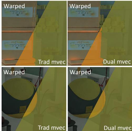
Figure 3. Visualizations of traditional motion vectors (Trad mvec) and dual motion vectors (Dual mvec) as well as the warped projections they produced. We set the opacity of motion vectors to 0.8 for intuition.
